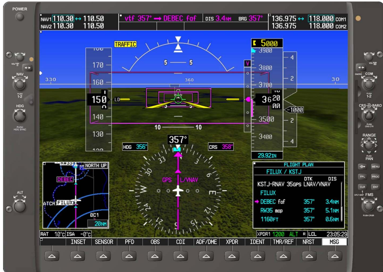
Figure 30 - Vertical deviation display with barometric approach vertical guidance
