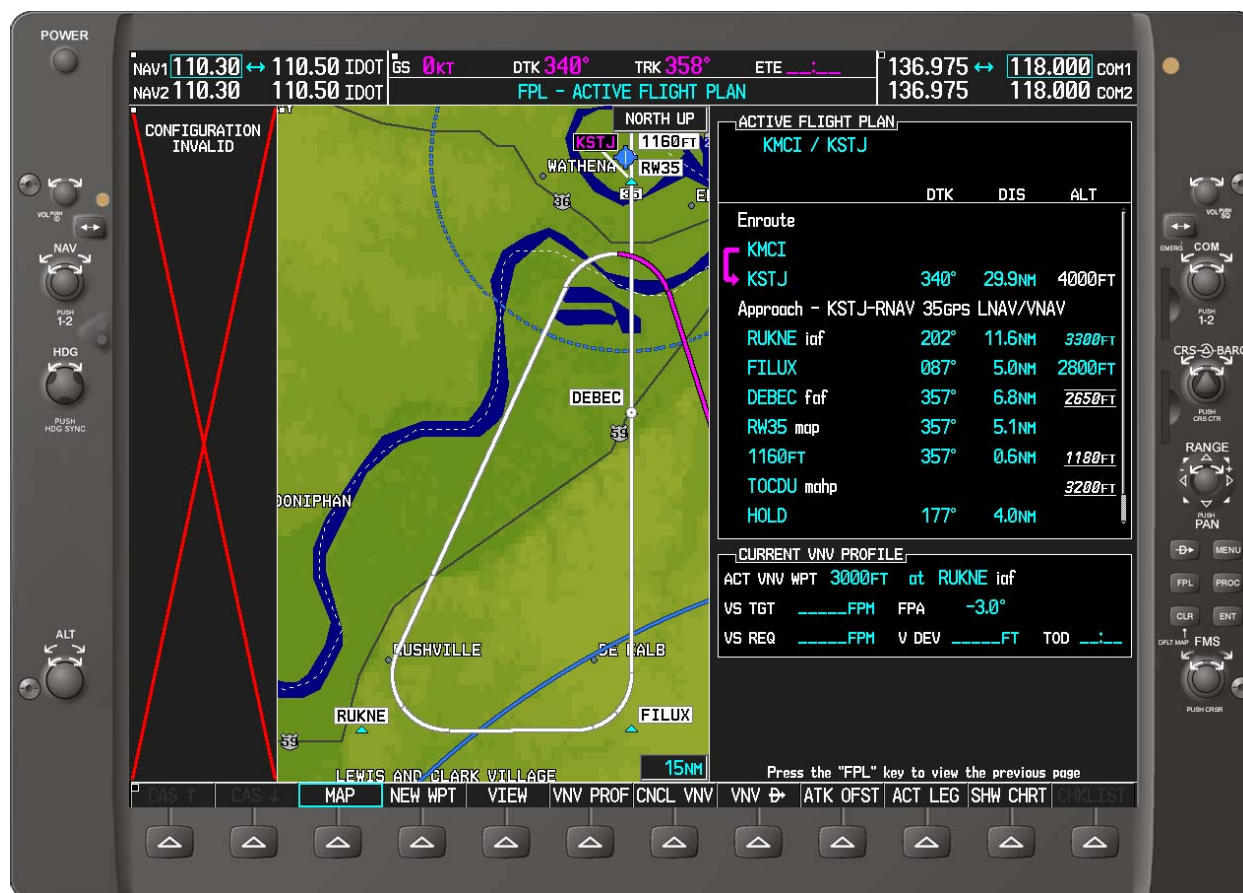
Figure 27- Display of Temperature-Compensated Altitudes
