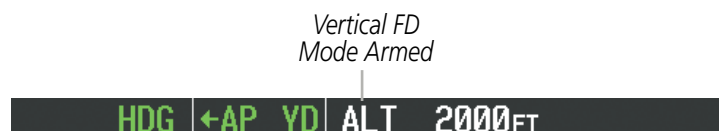
Figure 7-10 Vertical Flight Director Mode Armed
