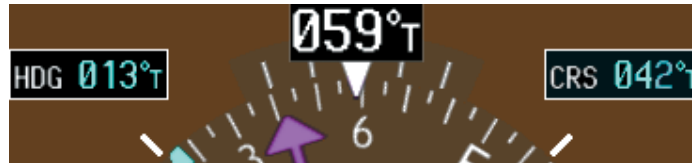
Figure 2-21 Heading and Course Indications (True)
