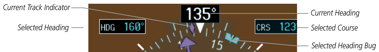
Figure 2-20 Heading and Course Indications
