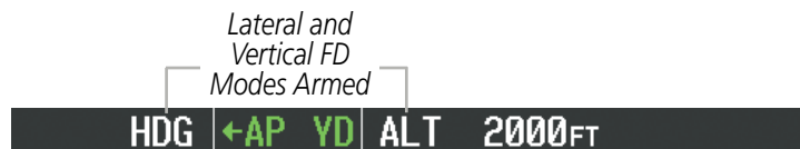
Figure 7-8 Lateral and Vertical Flight Director Modes Armed
