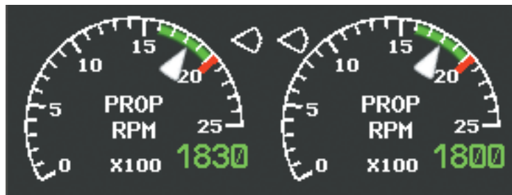
Figure 3-6 Propellers Out of Sync (less than 50 rpm)
