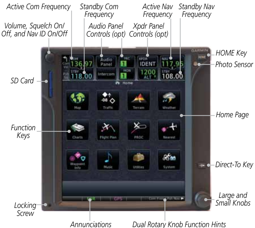
Figure 1-4 GTN 750 Front Panel
