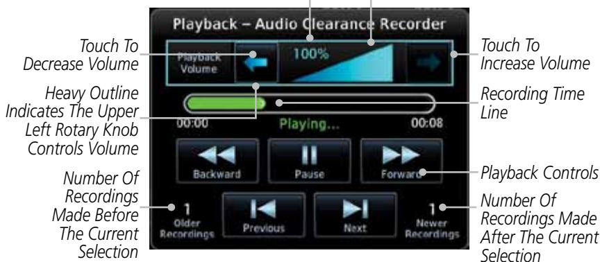
Figure 2-19 Audio Panel Playback Controls
