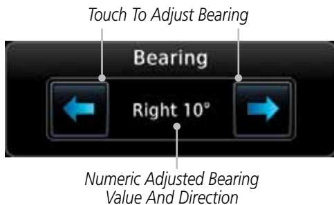
Figure 12-60 Bearing Line Adjustment
