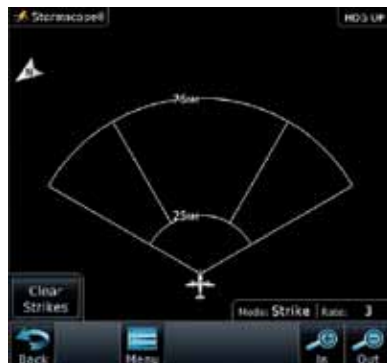
Figure 12-43 StormScope 360° and Arc Display Views
