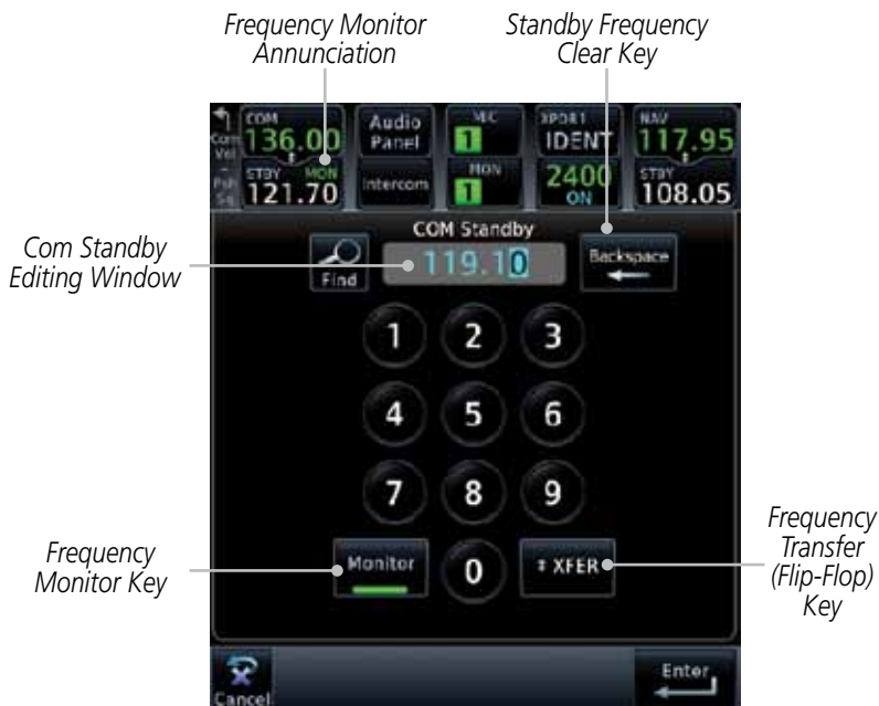
Figure 3-19 Com Frequency Monitoring
