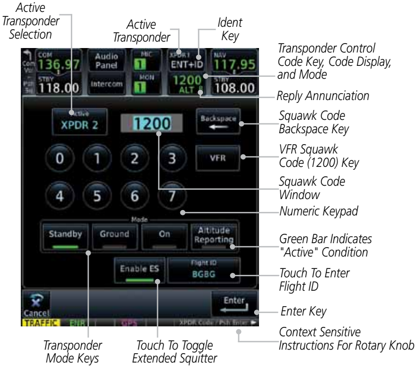
Figure 2-1 XPDR Control Display
