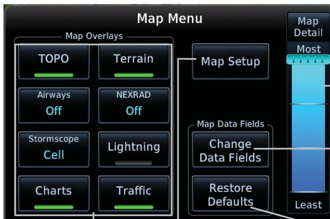
Touch to select which overlays are displayed. A green bar indicates the selection is enabled.
