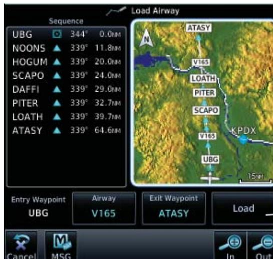
*Touch to load selected airway to flight plan.*
