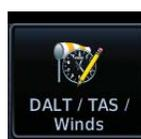
Touch to view calculations of density altitude, true airspeed, and wind.
