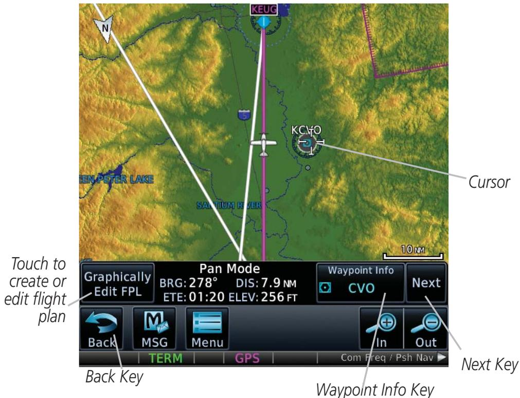
To exit Pan Mode, touch the **Back** key. To enter or edit a flight plan, touch the **Graphically Edit FPL** key.
