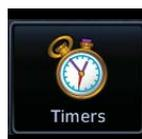
Touch to access timers. Generic Timer (count up or down), Flight Timer (set trigger to In Air or Power On), and Departure Time.
