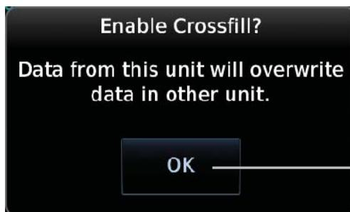
*Touch OK to enable crossfill with dual units.*
