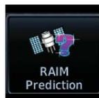
Touch to see the integrity of GPS satellite coverage at a particular waypoint at a particular time.
