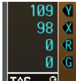
V Speed References on Airspeed Tape
