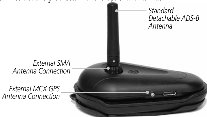
Figure 3-7 GDL 39 Antenna Connections
