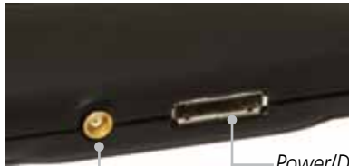
Figure 3-9 GDL 39 Antenna and Power/Data Port Connections
