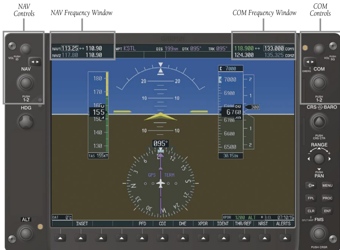
Figure 4-1 G1000 VHF NAV/COM Interface (PFD)
