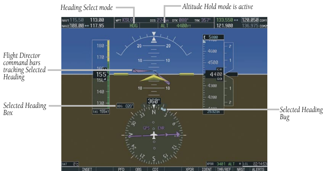
Figure 6-18 Heading Select Mode
