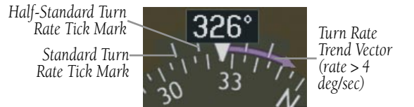
Figure 2-13 Turn Rate Indicator and Trend Vector
