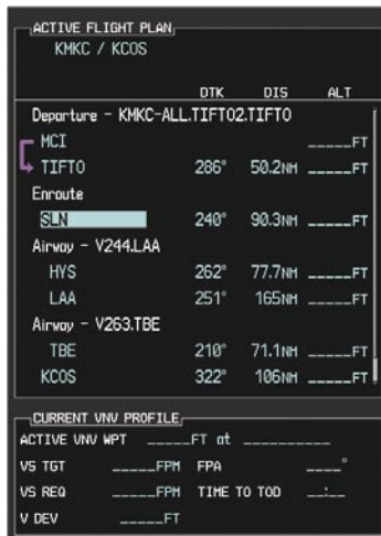
Figure 7-13 Begin Adding V4 to the Flight Plan
