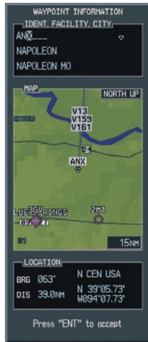
Figure 8-14 Load Airway Entry Point
