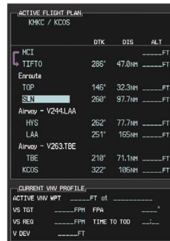
Figure 7-15 TOP Inserted into the Flight Plan
