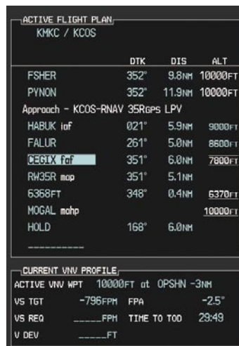
Figure 7-34 Vertical Guidance is Active to the FAF
