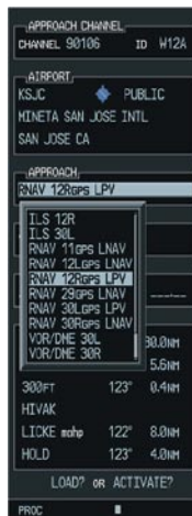
Figure 9-6 Selecting an Approach Procedure
