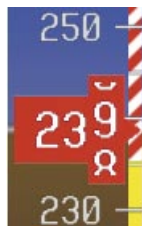
Figure 2-5 Red Pointer at V_{NE}
