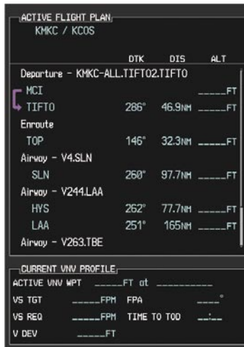
Figure 7-19 V4 is Loaded in the Flight Plan
