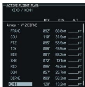
Figure 8-19 Airway Added to Flight Plan
