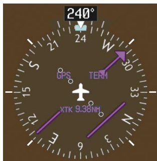
Figure 7-11 Assigned Heading of 240°
