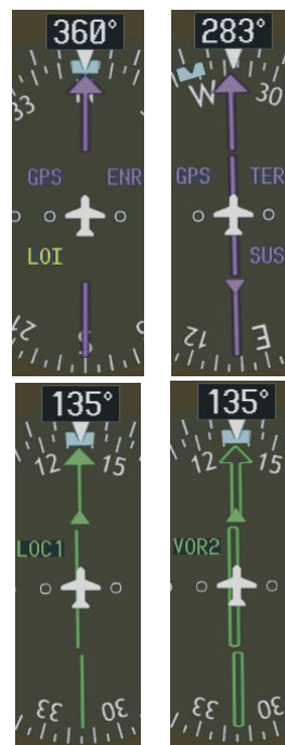
Figure 2-29 GPS LOI, GPS SUSP, LOC1 and VOR2
