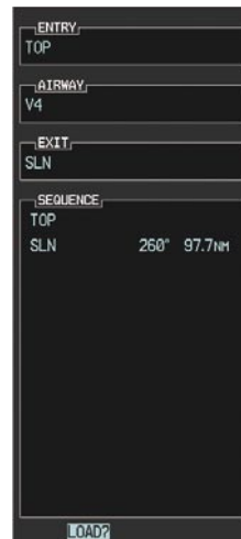
Figure 7-18 Ready to Load V4
