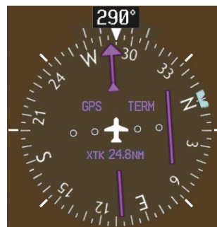
Figure 7-12 Assigned Heading of 290°
