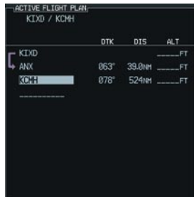
Figure 8-15 Airway Entry Point Loaded
