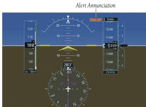
Figure 10-25 Alert Annunciation on the PFD
