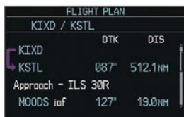
Figure 8-2 Active Flight Plan Window on the PFD
