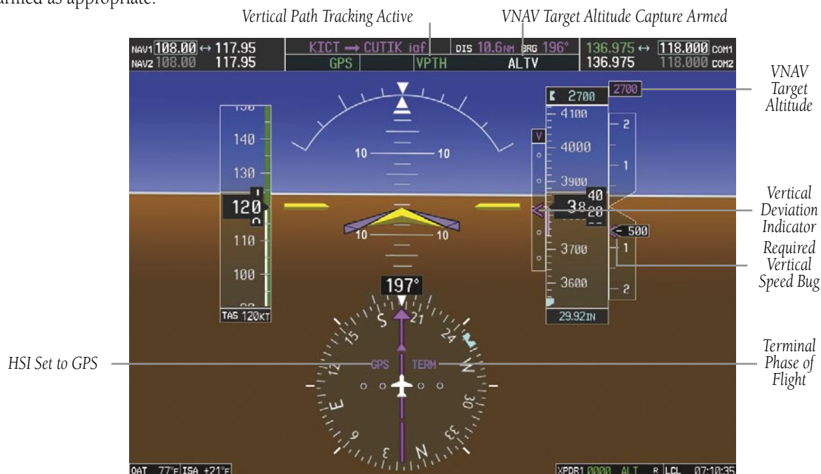
Figure 6-12 Vertical Path Tracking Mode
