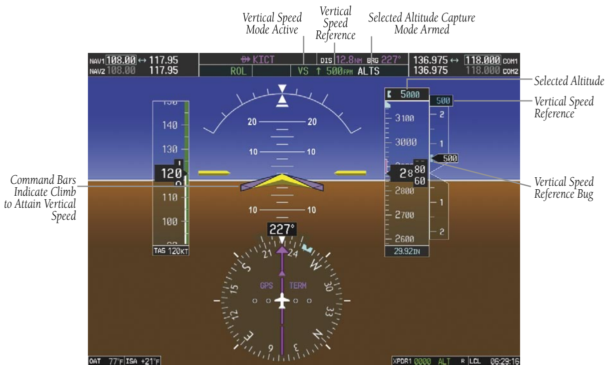
Figure 6-8 Vertical Speed Mode
