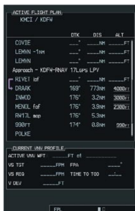
Figure 8-3 Active Flight Plan Page on the MFD
