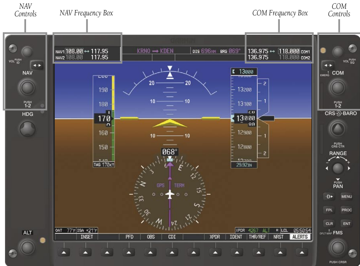
Figure 4-1 G1000 VHF NAV/COM Controls (PFD)
