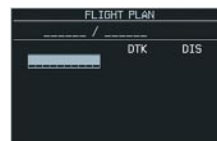
Figure 8-12 Creating Flight Plan on the PFD
