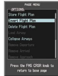
Figure 8-8 Invert Flight Plan
