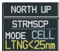
Figure 10-5 Lightning Display Range Annunciation
