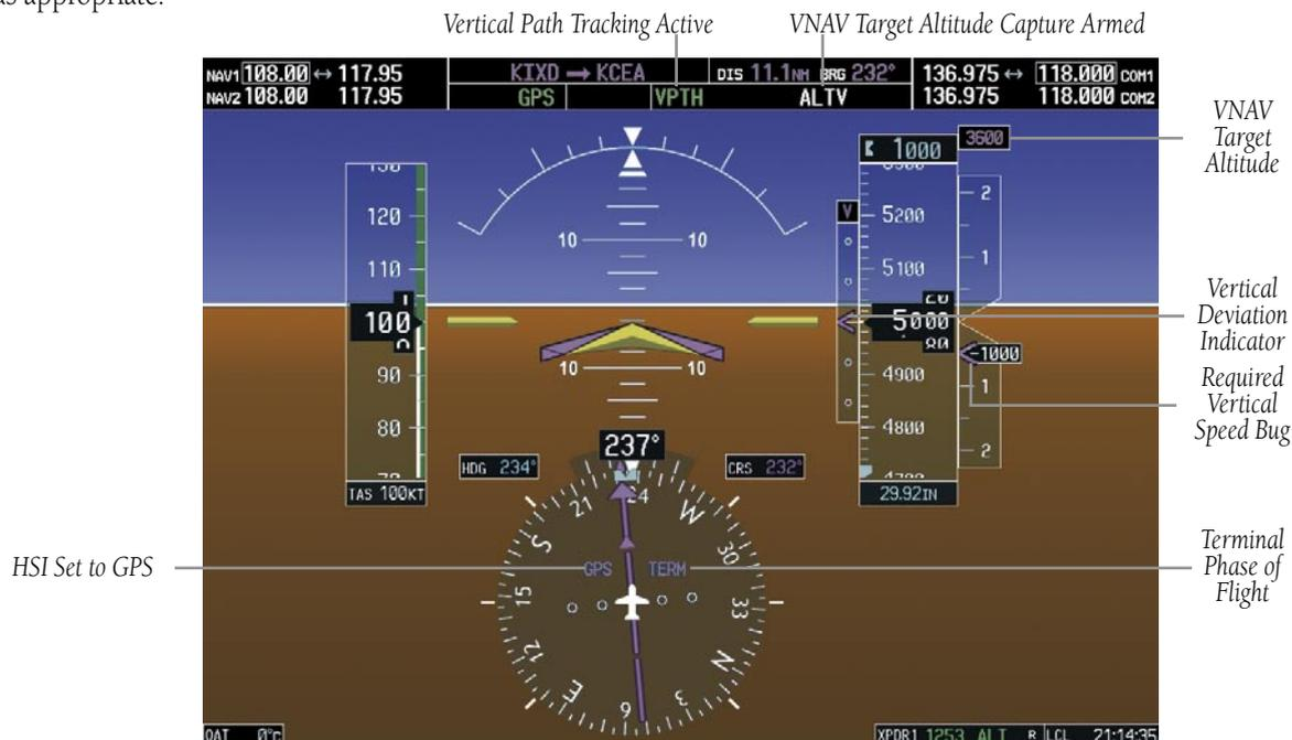
**Figure 6-12 Vertical Path Tracking Mode**
