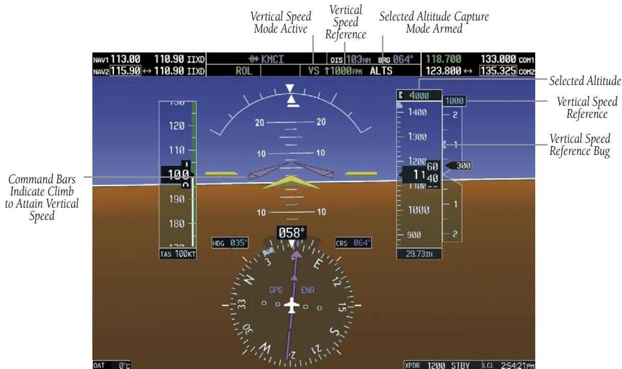
Figure 6-8 Vertical Speed Mode
