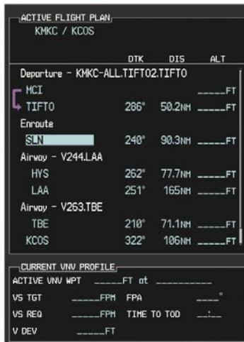
Figure 7-13 Begin Adding V4 to the Flight Plan
