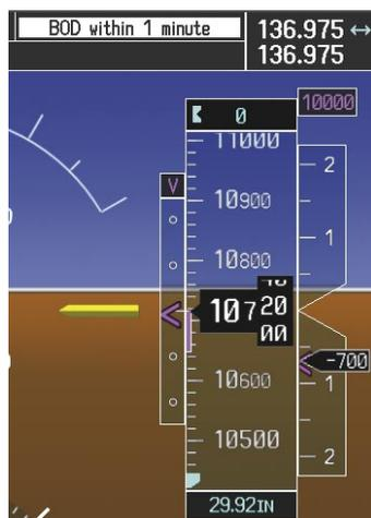
Figure 7-39 Approaching Bottom of Descent (BOD) at OPSHN
