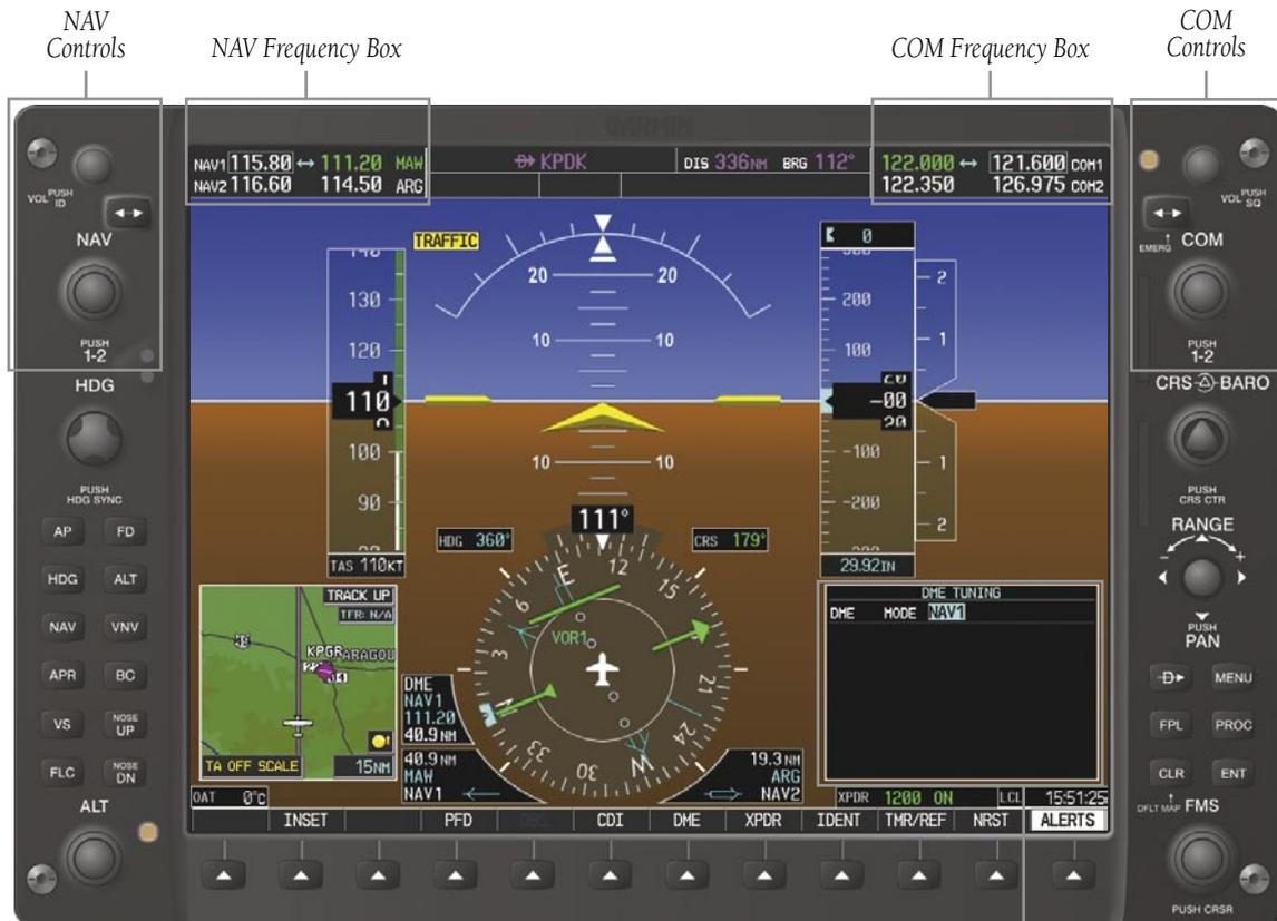
Figure 4-1 G1000 VHF NAV/COM Interface (PFD shown)
