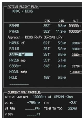
Figure 7-34 Vertical Guidance is Active to the FAF
