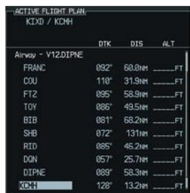
Figure 8-18 Airway Added to Flight Plan
