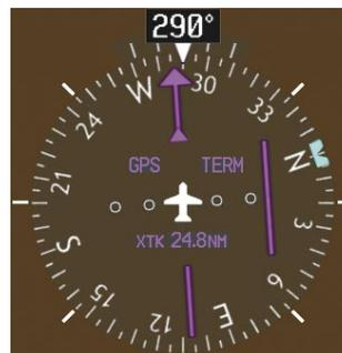
Figure 7-12 Assigned Heading of 290°
