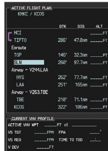
Figure 7-15 TOP Inserted into the Flight Plan
