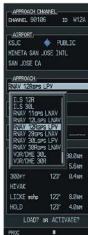
Figure 9-6 Selecting an Approach Procedure
