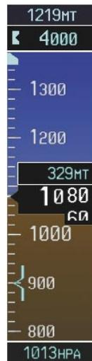
Figure 2-9 Altimeter (Metric)
