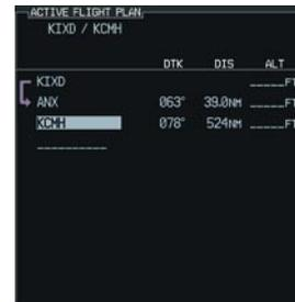
Figure 8-15 Airway Entry Point Loaded
