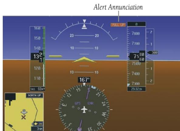
**Figure 10-27 TAWS Alert Annunciation on the PFD**
