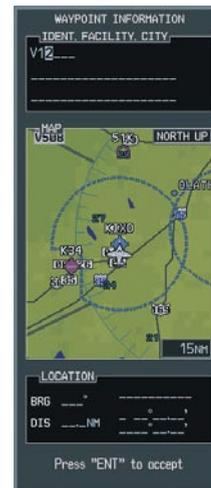
Figure 8-16 Enter Airway Identifier
