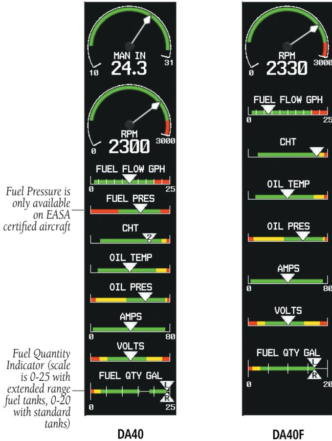
**Engine Instrument Display on the MFD**
