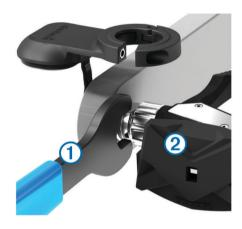
**NOTE:** The spindle and crank for the left pedal has a left-handed (reverse) thread.
