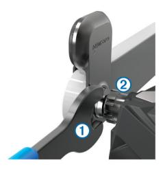
**NOTE:** The spindle and crank for the left pedal has a left-handed (reverse) thread.
