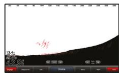
To help give you time to avoid collisions with submerged obstacles, FrontVü shows underwater obstructions within a 300' range as you approach them in real time<sup>1</sup>.
