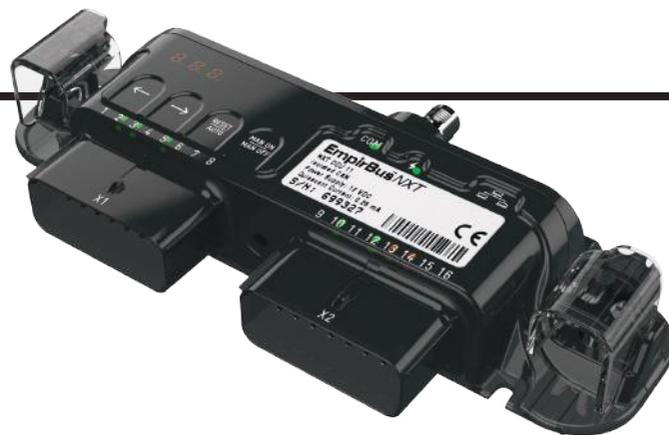
With multiple input capabilities and ranges the DCM is an extremely versatile and cost effective means to interface signals to the system and when combined with the powerful NXT software complex monitoring and control systems are easily realized in practice.
