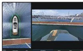
A visual bumper feature helps the captain see when docks, piers or other objects breach preset barrier limits around the boat.
