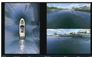
The 360-degree video feed integrates with compatible Garmin chartplotters or MFD helm displays. Each camera view can also be monitored individually.
