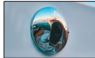
Thru-hull OEM installation offers secure fit and calibration of the Surround View Camera System. For easy maintenance, any of the cameras can be replaced externally.
