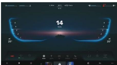
EmpirBus systems feature fully customizable layouts and graphics that allow for every circuit switch or monitor to be shown in any configuration with a simple drag-and-drop graphic interface builder. Screens can even be personalized by uploading boat images.
