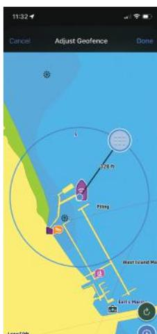
Be the first to know if a security sensor has been triggered, or if your boat has been moved. The internal GPS sensor updates every 15 or 30 minutes, depending on power status, and will send text alerts<sup>1</sup> if your boat leaves the geofenced area.
