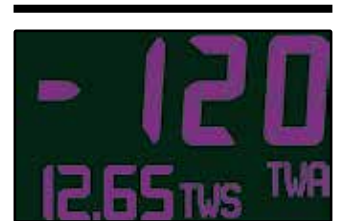
True wind angle and true wind speed
